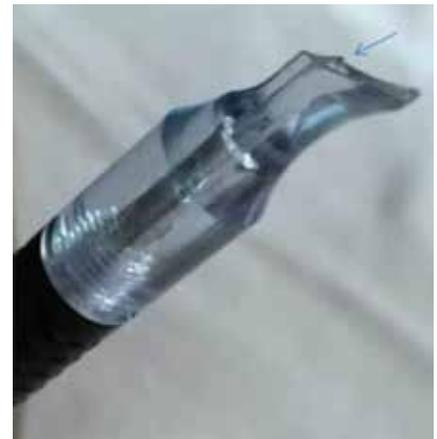
Figure 5: Side view of IRIS G-probe showing protruding fibre optic (0.7mm) from foot plate.
