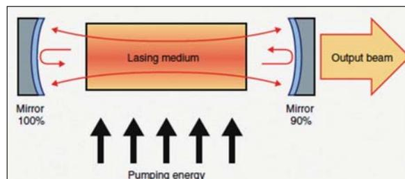
**Figure 1:** Laser typically consists of the energy source (pump), the lasing medium, and the optical cavity with a partially transparent front mirror.
