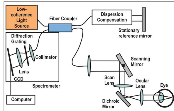
Figure 3: Optics of Spectral Domain OCT.
